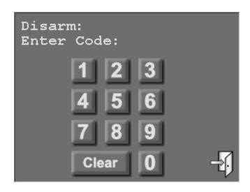
Enter your four-digit code. If you make a mistake, press the [Clear] button and start over or press the [exit] button to return to the previous page. After the last digit of a valid code is entered, the system will perform the desired task.
