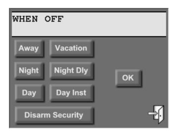
Press the desired security mode button. Once complete, press the [OK] button to save the security mode. Note: The program will activate at the end of the "exit delay" (if applicable).
