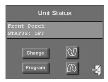
Press [page down] to display the next item and press [page up] to display the previous item. Press the [Change] button to change the status of the selected device.
