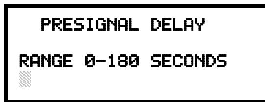
Pre-signal Delay Screen
