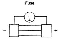
TO TEST BATTERY VOLTAGE: Measure voltage across battery terminals.
